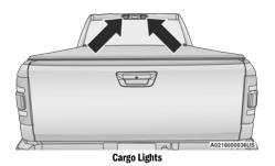
When the vehicle is stationary, these lights can also be turned on using the switch located just inside the pickup box, on the lower part of the bed light lens. A telltale will illuminate in the instrument cluster display when these lights are on. Pushing the switch a second time will turn the lights off.
