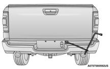
Inserting The Extension Tubes Into The Access Hole
