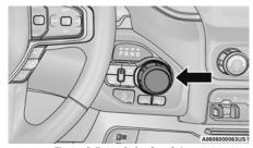
Electronic Transmission Gear Selector
