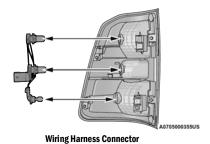
Rotate the bulb socket counterclockwise a quarter turn to unlock it from the housing.
