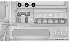
Integrated Trailer Brake Module (ITBM)
