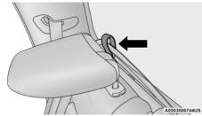
Tether Strap Through Outboard Tether Strap Loop
