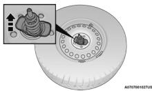
**Reinstalling The Retainer**
