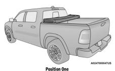
(Front Latches Latched And Stowage Straps Secured)
