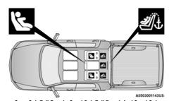
Crew Cab Full Bench, Quad Cab Full Bench And Quad Cab 60/40 Split Bench LATCH Positions
