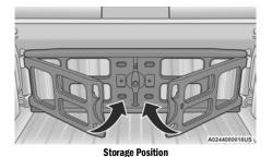
The outboard ends should be positioned in front of the cargo tie-down loops.
