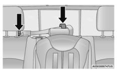
Tether Strap Through Center Tether Strap Loop And Attached
