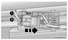
**Connected Wiring Harness**
