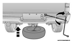
**Reinstalling The Flat Or Spare Tire**
