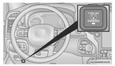
Instrument Panel Power Inverter Switch
