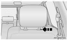
**Head Restraint Adjustment Button Location**
