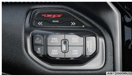
Four-Position/On-Demand Transfer Case
