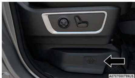
Pull Jack Access Cover From Front
