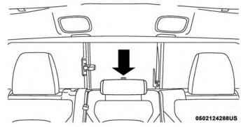
Center Tether Anchorage Over Head Rest
