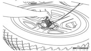
Reinstalling The Retainer
