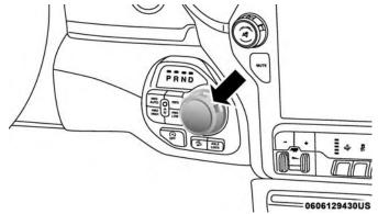
**Electronic Transmission Gear Selector**
