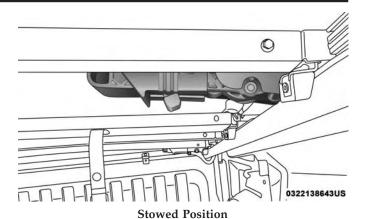
4. Lift up on the Tonneau Cover and fold it back onto the second panel.
