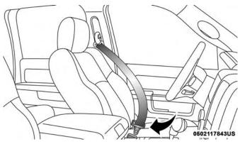
**Inserting Latch Plate Into Buckle**
