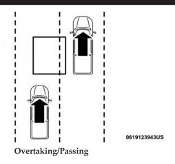
The BSM system is designed not to issue an alert on stationary objects such as guardrails, posts, walls, foliage, berms, snow banks, car washes etc. However, occasionally the system may alert on such objects. This is normal operation and your vehicle does not require service.
