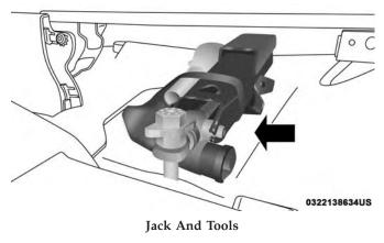
Release the tool bag straps from the jack and remove tools from bag.
