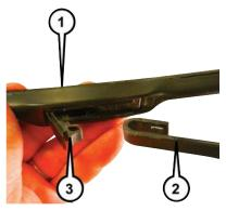
Wiper Blade Removed From Wiper Arm
