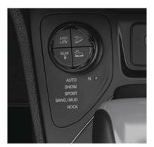
2-Speed 4x4 Switch (with Rear Lock)
