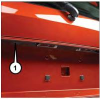
1 — Electronic Liftgate Lock/Unlock Pad
