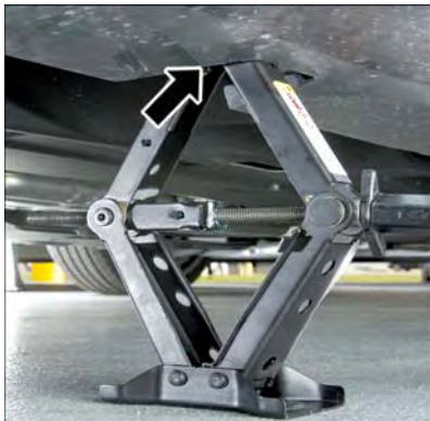
Front Jacking Location Engaged
