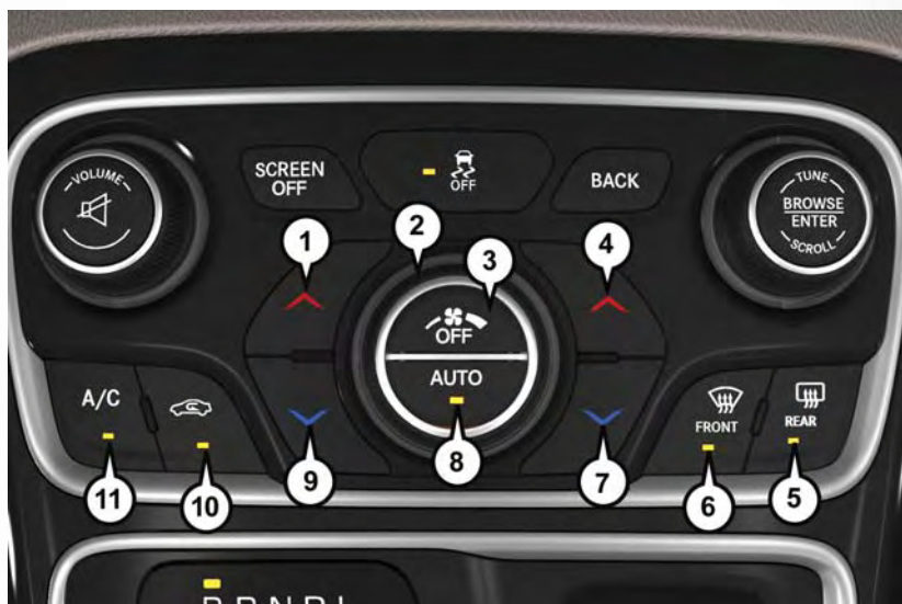
Automatic Climate Controls
