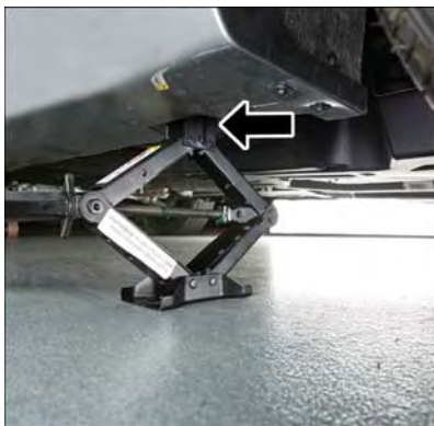
Rear Jacking Location Engaged
