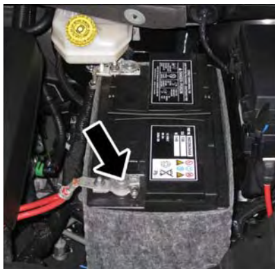
Positive Battery Post
