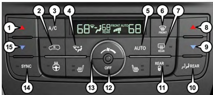
Three Zone Automatic Temperature Controls (ATC)
