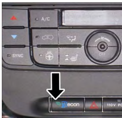
ECON Switch Location
