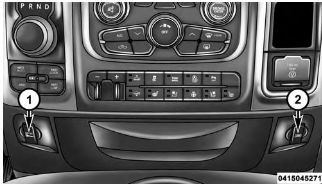
Power Outlets — Center Stack
