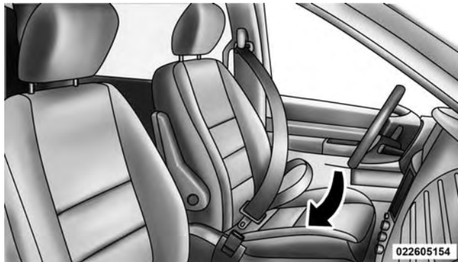
Inserting Latch Plate Into Buckle
