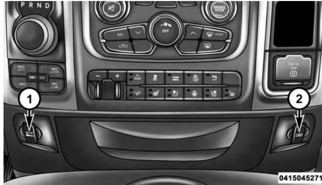
Power Outlets — Center Stack
