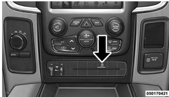
STOP/START OFF Switch
