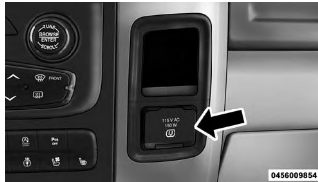
Power Inverter Outlet
