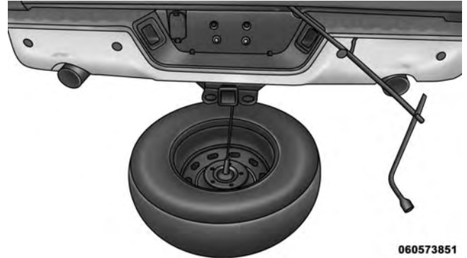
Pulling The Spare Tire Out
