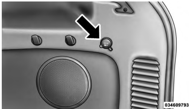
Rear Power Outlet
