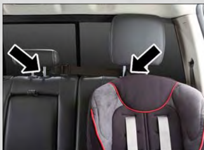
Tether Strap Through Outboard Tether Strap Loop And Attached To Center Tether Strap Loop
