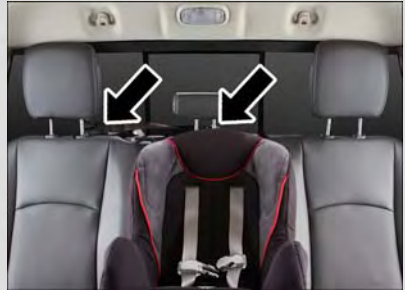
Tether Strap Through Center Tether Strap Loop And Attached To Outboard Tether Strap Loop
