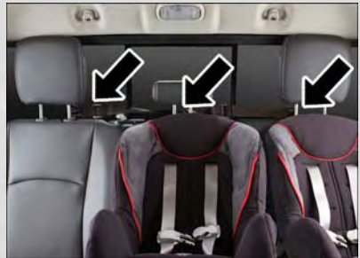
Left Outboard And Center Seating Position Shown
