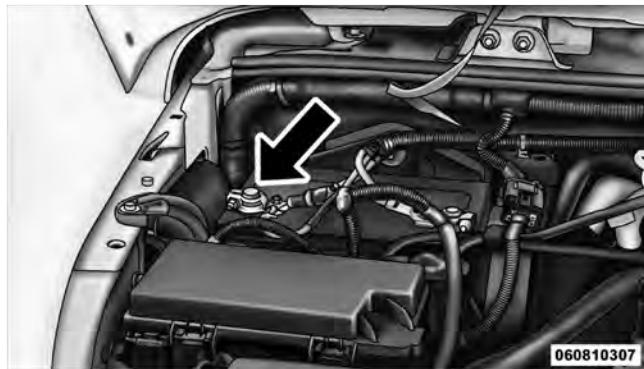
Positive Battery Post
