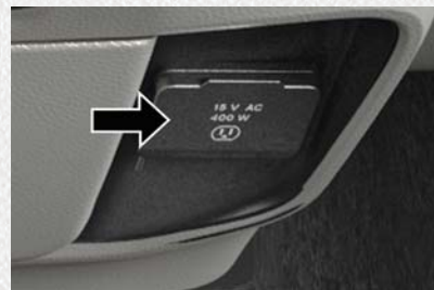
Center Stack Power Inverter
