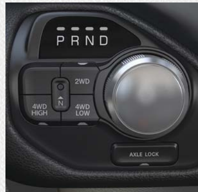
Four-Position/On-Demand Transfer Case — Eight Speed Transmission Only
