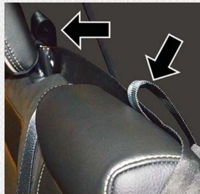
Tether Strap Through Center Tether Strap Loop And Attached To Outboard Tether Strap Loop
