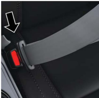
**Inserting Latch Plate Into Buckle**
