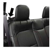
Rear Head Restraint Folding Strap Location
