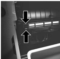
Air Filter Retaining Tabs
