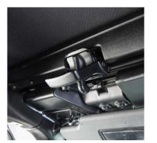
Header Latch Disengaged
