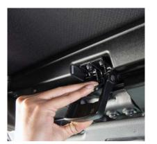
Squeeze Latch Plate And Pull Handle Upward
