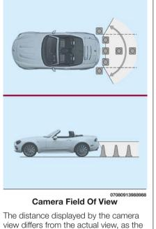
The distance displayed by the camera view differs from the actual view, as the rear parking camera is equipped with a special lens.
