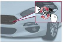
Installing Front Towing Eye
