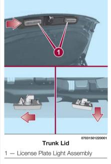
3. Turn the socket and bulb assembly counterclockwise and remove, remove bulb.
