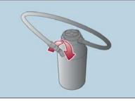
Install Injection Hose To Sealant Bottle **Note:** The remaining sealant in the hose may spray out when the hose is removed. Remove the hose carefully because you may not be able to remove the sealant contacting clothing or other objects.
