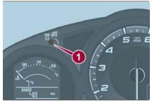
Odometer/Trip Reset Button
