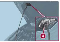
Inserting Support Rod Into Hole
