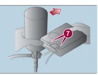
Sealant Bottle Into Air Compressor
