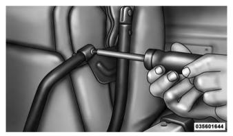
4. Disconnect the knuckles from the left and right metal pivot brackets. Remove the soft top from the vehicle and store in a clean, dry location.
