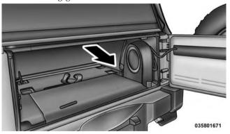
will stay on the rear window. Pull down on the rear window to disengage it from the zipper on the top cover.
