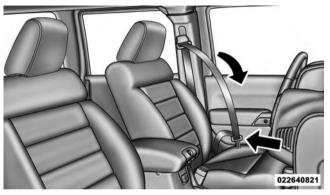
Pulling Out The Lap/Shoulder Belt Latch Plate
