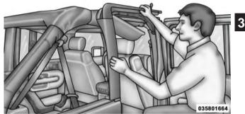
3. Position the top of the door frame against the metal sport bar and press onto the side bar making sure not to pinch the material of the sports bar covers and to ensure it is properly positioned on the seal above the front of the rear door.
