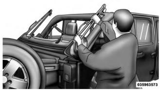
20. Tuck the fabric and the check straps between the bows as far inside as possible. This will keep any portion of the top from flapping outside of the vehicle.
