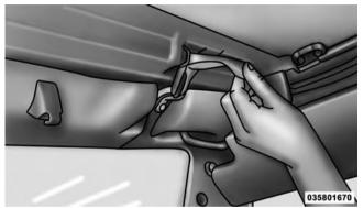
4. Release the sail panel retainers from the body side 5. As you be channel at the rear corners of the vehicle. that they
