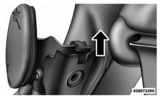
8. Remove the soft top from the vehicle and store in a clean, dry location (another person may be needed to help with this operation).
