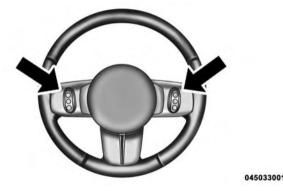
Remote Sound System Controls (Back View Of Steering Wheel) The right-hand control is a rocker-type switch with a push-button in the center and controls the volume and mode of the sound system. Pressing the top of the rocker switch will increase the volume, and pressing the bottom of the rocker switch will decrease the volume.
