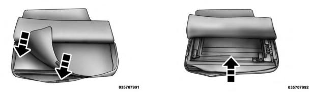
Insert the left-side Freedom panel into the bag with the Unfold the outer flap and zip the Freedom bag closed. latches facing upward.
