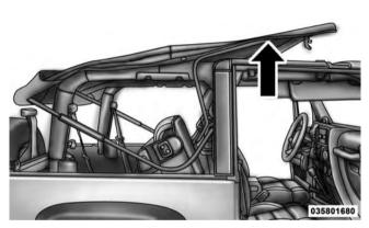
18. Tuck the fabric and the check straps between the bows and as far inward as possible. This will keep any portion of the top from flapping outside of the vehicle.
