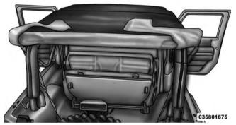
**NOTE:** When releasing the sail panel retainers, it is helpful to pull down on the rear roof bow.
