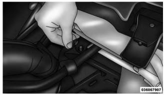
10. Remove the swing gate bar (black metal bar for bottom of rear window) and set aside.
