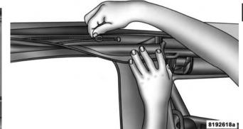
13. Insert the front retainer of the window into the door channel, making sure the retainer is fully seated and properly positioned on the door frame. Failure to do so can result in wind and water leaks or damage to the window.
