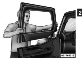
**Upper Half Door Window** Grasp the half door window and pull upward.
