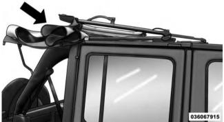
17. Release the side bows by pressing down on the latch above the front of the rear door. Push the top rearward to disengage. Repeat this step on the other side.
