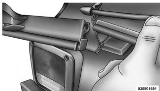
13. Locate the black swing gate bar. Slide the swing gate bar over the receiver at the bottom inside of the rear window. The spongy part of the seal should be down and pointed outward to seal with the swing gate when closed.
