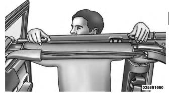
8. Loosely install both knobs beginning with the front knob (long knob). Then, install the middle knob (short knob) through the front and rear door frames and screw into the top of the B-pillar.
