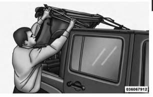
19. Gently slide the side bows off the door frame track and lower the top down into the vehicle.
