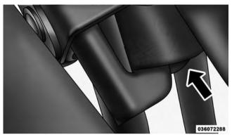
8. Using the plastic reinforcement as a handle remove the tether strap from the bracket hook by sliding strap up off hook and slide down the side bow (both sides).
