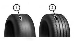
1 — Worn Tire 2 — New Tire These indicators are molded into the bottom of the tread grooves. They will appear as bands when the tread depth becomes 1/16 in (2 mm). When the tread is worn to the tread wear indicators, the tire should be replaced. Refer to replacement tires in this section for further information.
