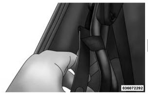
5. The tether strap **must** be hooked onto the pivot bracket prior to removal of soft top from vehicle (both sides).
