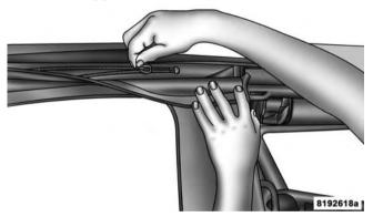
7. Insert the front retainer of the window into the door channel, making sure the retainer is fully seated and properly positioned on the door frame. Failure to do so can result in wind and water leaks or damage to the window.
