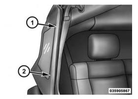
1 — Incorrect Insertion 2 — Correct Insertion 14. Insert the retainer along the bottom edge of the window into the bottom side channel, beginning at the front and working to the rear of the vehicle. Finish by closing the zipper completely and attaching the Velcro® along the top and rear of the window. Repeat this step for the opposite side.
