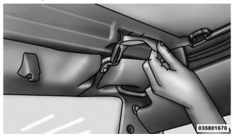
7. If the swing gate brackets were removed, install them by hooking the rear edge of the bracket on the interior side of the body channel. Then, rotate it rearward and over the channel until it snaps onto the exterior part of the rail. To be properly located, the bracket must only be clipped to the shortened rail edge.
