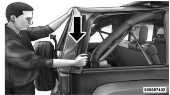
3. Rotate the header forward.
