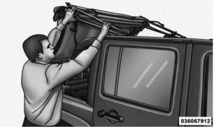
6. Ensure that the top locks into the Sunrider® locking mechanisms that are located above the front of the rear doors.
